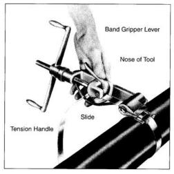
Place band in open slot of tool nose and in slide. With thumb on band gripper lever, apply tension by turning handle of tool. After tension is created, it is no longer necessary to hold band gripper lever as it locks itself under tension.
