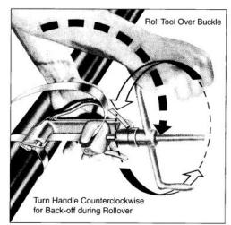
Roll tool over buckle, backing off with tension handle throughout entire rolling operation. Failure to back off with tension handle throughout entire course of roll may result in breaking of band. There is no loss of tension as band released is used up in the band.
