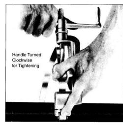
Place finger on the band at buckle bridge while tensioning with tool handle. When you feel the band stop moving through buckle as you are turning handle, maximum pressure is being exerted by the band around object being clamped. Stop turning handle.
