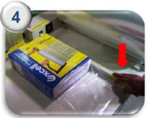
Press the **sealing arm** firmly down and hold until the red light switches off. The sealed product should pull away easily.
