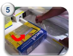
Rotate and repeat the sealing on the open side ,tearing the excess plastic away as the sealing light switches off.
