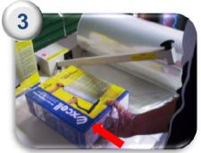
Pull a length of film out and insert the **product** between the two pieces of film
