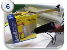
Apply the **heat gun** to all sides of the product. The heat will shrink the film firmly around the product.
