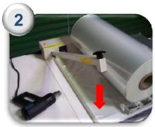
Part it with the **separating plate** and pull a length under the **sealing arm**. Press the sealing arm down to seal the film closed.
