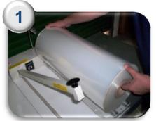
According to the micron of the film set the **control dial** (inset) between 5 and 8. Place the roll of **POF centerfold film** on the **rollers**.
